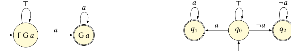
(a) A nondeterministic Büchi automaton for the absolute liveness specification FG a , used as a counterexample to the “only-if” direction of Lemma 3.4.
