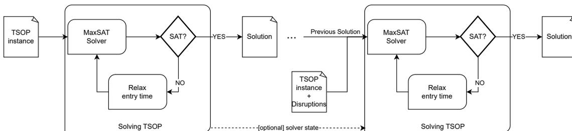
Figure 4: Overview of the solution to solve TSOPuD.
