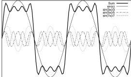
Figure 1: Fourier series approximations for a square wave, showing contributions from the first two and a the first four nonzero harmonics.
