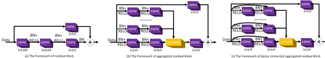
Figure 2: Architecture of the residual block and its extensions. (a) refers to the original residual block, and (b) the aggregated residual block, and (c) the dense connected aggregated residual block.)
