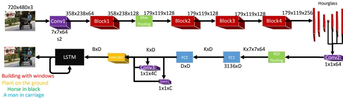
Figure 1: Illustration of the Framework. The numbers between volumes are the size of the tensor.  $K$  is the number of proposals that are obtained from an hourglass network,  $D$  is the hidden unit dimension,  $C$  is the object class number (including the background), and  $B$  objects with the highest confidence scores are selected and fed into LSTMs.
