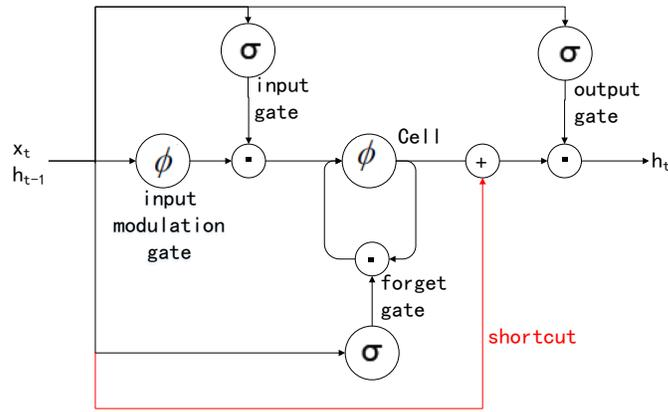
Figure 4: Architecture of LSTM and Residual LSTM. LSTM has no shortcut, while Residual LSTM has a shortcut.
