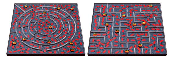
Figure 3: Examples of roadmaps and triangulation of the obstacle-free area  $\mathcal{W}_{\text{free}}$ .
