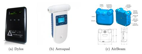
Figure 1: Examples of portable devices that measure air quality in terms of atmospheric particulate matter (PM).
