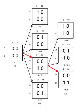
Figure 5: Schematic representation of an SLGS Algorithm example
