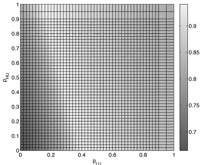
Figure 16: Load factor for different proportions of low-end and high-end users adopting storage.
