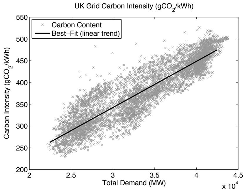
Figure 3: Half-hour UK grid carbon intensity plotted against total demand for August and September 2009 illustrating the correlation between carbon intensity and demand.
