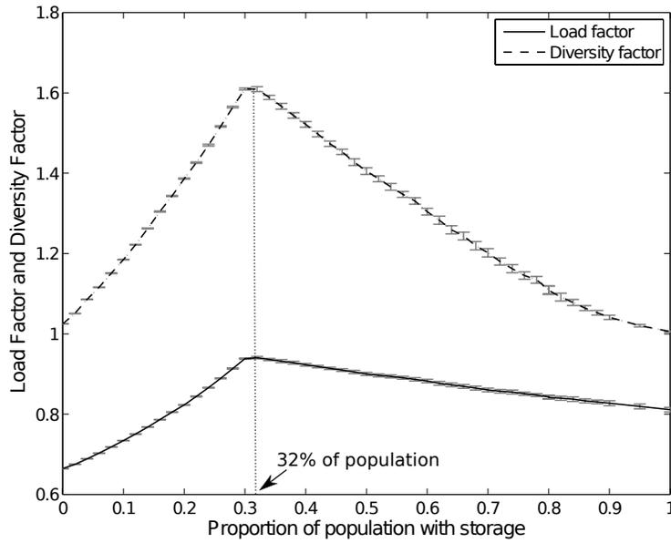
Figure 11: Grid efficiency (i.e., the load factor and the diversity factor) for different proportions of the population using storage.
