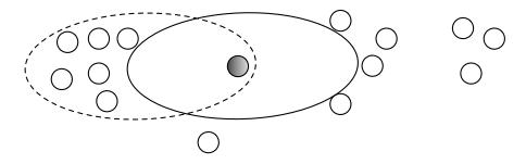
Figure 2: The behavior of the sum heuristic vs. that of the progress heuristic. The solidline ellipse indicates the area covered by a search using the sum heuristic. The dotted-line ellipse marks the area searched using the progress heuristic.
